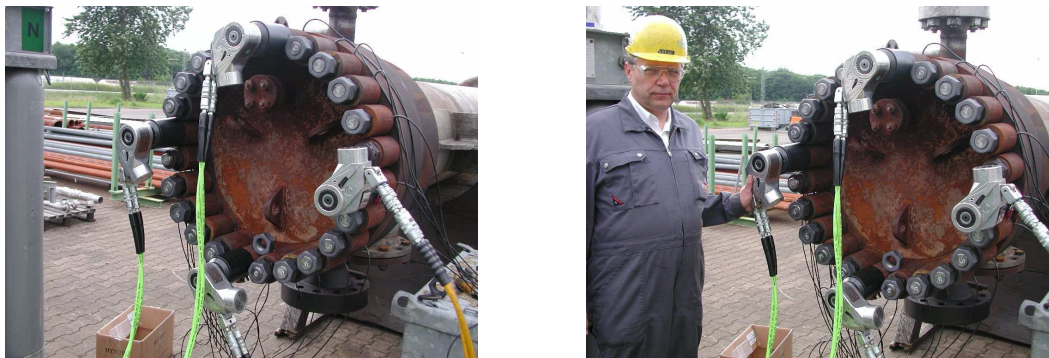
Figure 12: Start position of the Hytorc Avanti 5 tools
